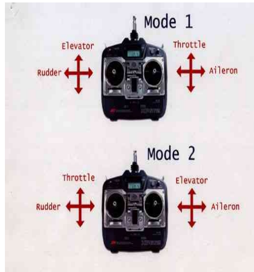
Figure 6.8: Conventional modes of an RC transmitter [51]
